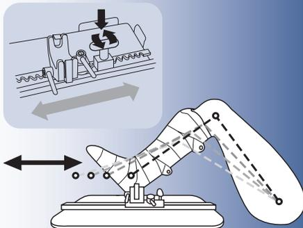
The Ratchet allows the Yoke Assembly to be moved in a precise gradual manner, the length of the Track. For faster adjustments, downward pressure on the Ratchet Handle releases the Yoke Assembly which then can be easily slid the length of the Track.
