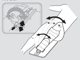
Loosening the Tilt Bar allows the knee to be tilted in either direction. Tightening the bar locks the Yoke System in the desired position.
