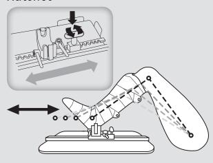
Turning the Ratchet allows the Yoke Assembly to be moved in a precise gradual manner, the length of the Track. For faster adjustments, downward pressure on the Ratchet Handle releases the Yoke Assembly which then can be easily slid the length of the Track.
