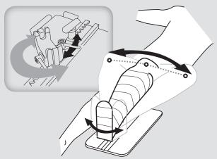
Loosening the Rotation Bar allows the knee to be rotated in either direction. Tightening the bar locks the Yoke System in the desired direction.
